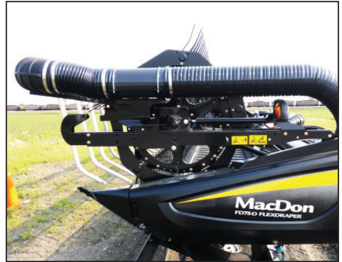
Figure 64: Left side view of hose routing
